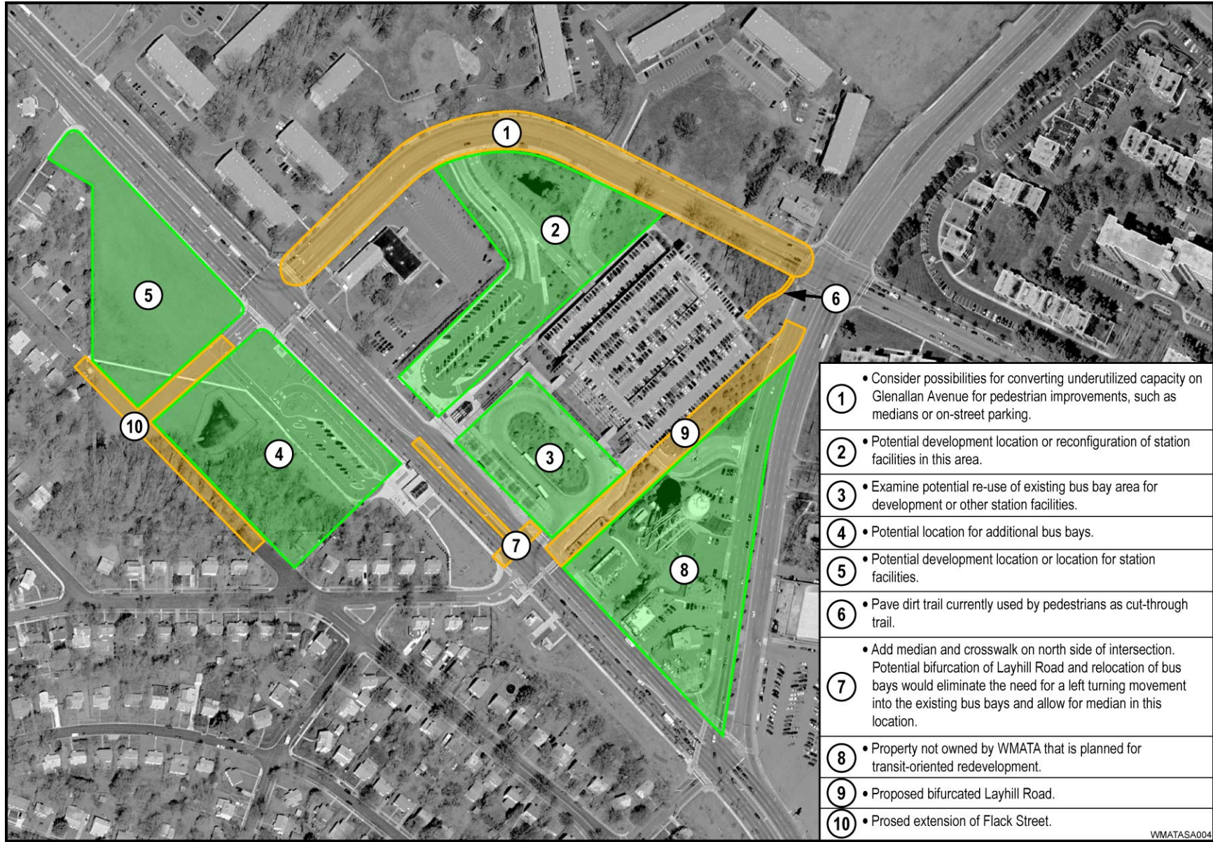
Figure E-3: Glenmont Station – Access Improvements
