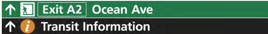
Figure 3.2.5.1: Two messages in the same direction. The Exit message (green background) always appears on top. The messages are separated by a white horizontal rule.
