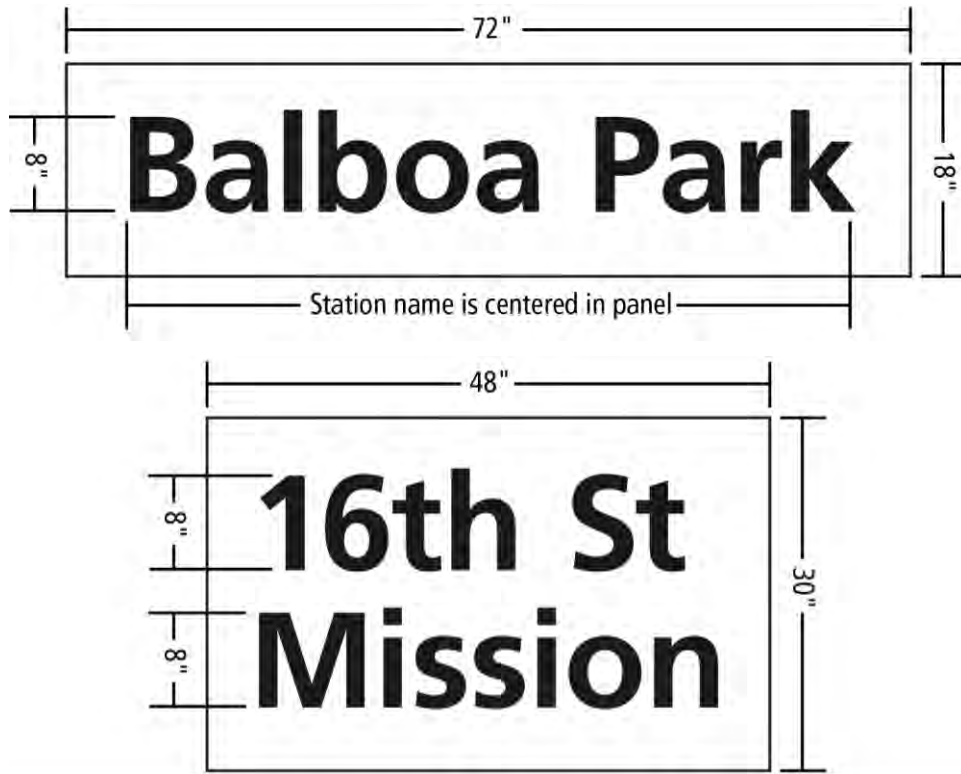
Figure 3.5.2.1: Trackway station identification signs. Type and arrows are black on a white background. Size of panel varies by length of message.
