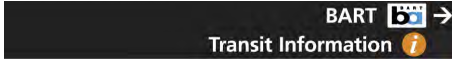
Figure 3.2.6.2: Two messages in the same direction on the same background color. Only one arrow is shown, and no separating rule.
