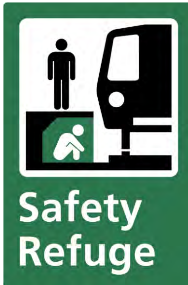
Figure 5.5.1.2: Safety Refuge sign (trackway) 12 x 18 in.
