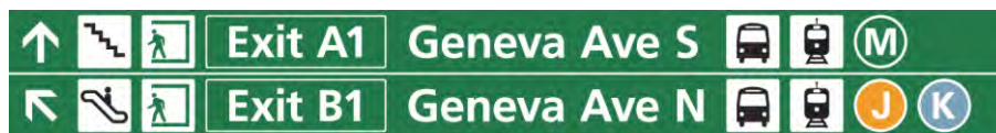
Figure 3.2.2.2: In this example, the destination at top is located straight ahead along a corridor. The second destination is a vertical access point (escalator) immediately to the left of the viewer — the “up left” arrow is used to indicate this (see Figure 3.1.2.3).
