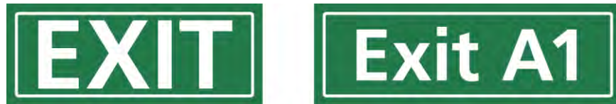
Figure 3.3.1.2: The word EXIT and the alphanumeric designation (if present) are enclosed in a white outline box in order to separate them from the text message.
