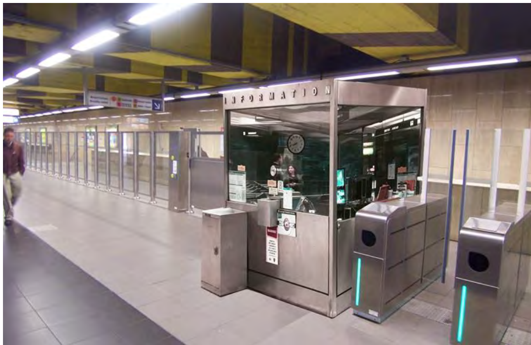
Figure 4.1 – Example of barrier between paid area and non-paid area, with a station agent booth adjacent to service gate and fare collection gates.
