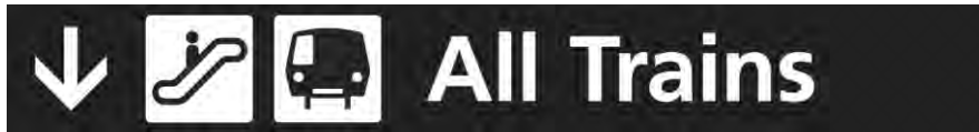
Figure 3.2.2.3: This sign would be used at the top of an escalator leading down to the platform. Message is left-aligned by default. The BART Train symbol follows the vertical access symbol.
