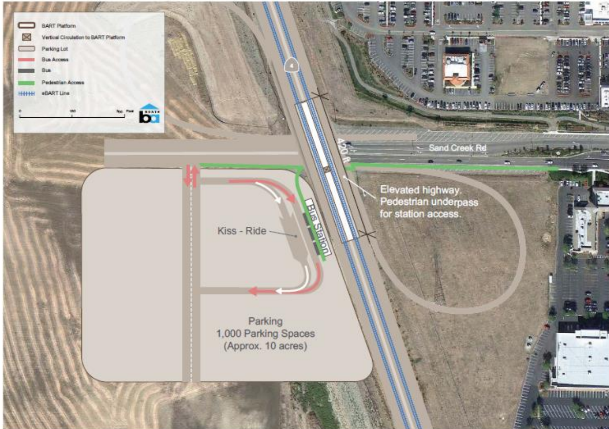
Figure 28 – eBART Sand Creek Road Station Area
