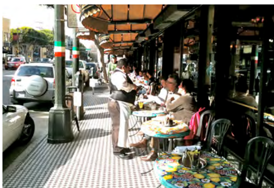
Wide sidewalks should allow space for sidewalk vending and outdoor seating, street amenities, and a six-foot clear pedestrian walkway.
