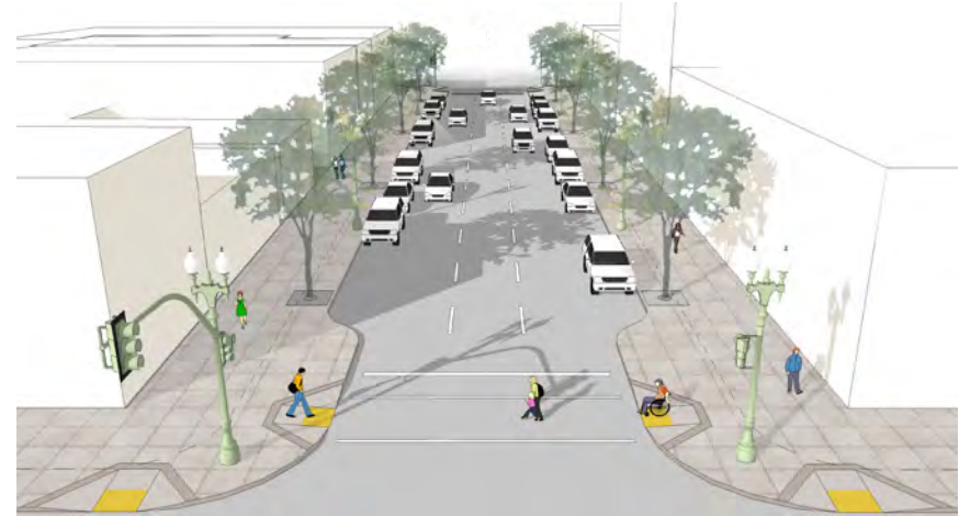
Phase II Option B: Sidewalk widening with lane reduction (if it is determined that conversion is not feasible).
